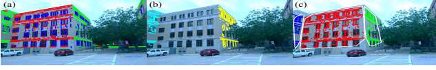
Fig. 4: Extracting PBFs (Best viewed in color). (a) Feature points associated to vanishing direction of neighboring (color-coded) horizontal line segments. (b) Homography clustering applied to feature points with same vanishing direction. (c) Convex hull for each homography cluster.
